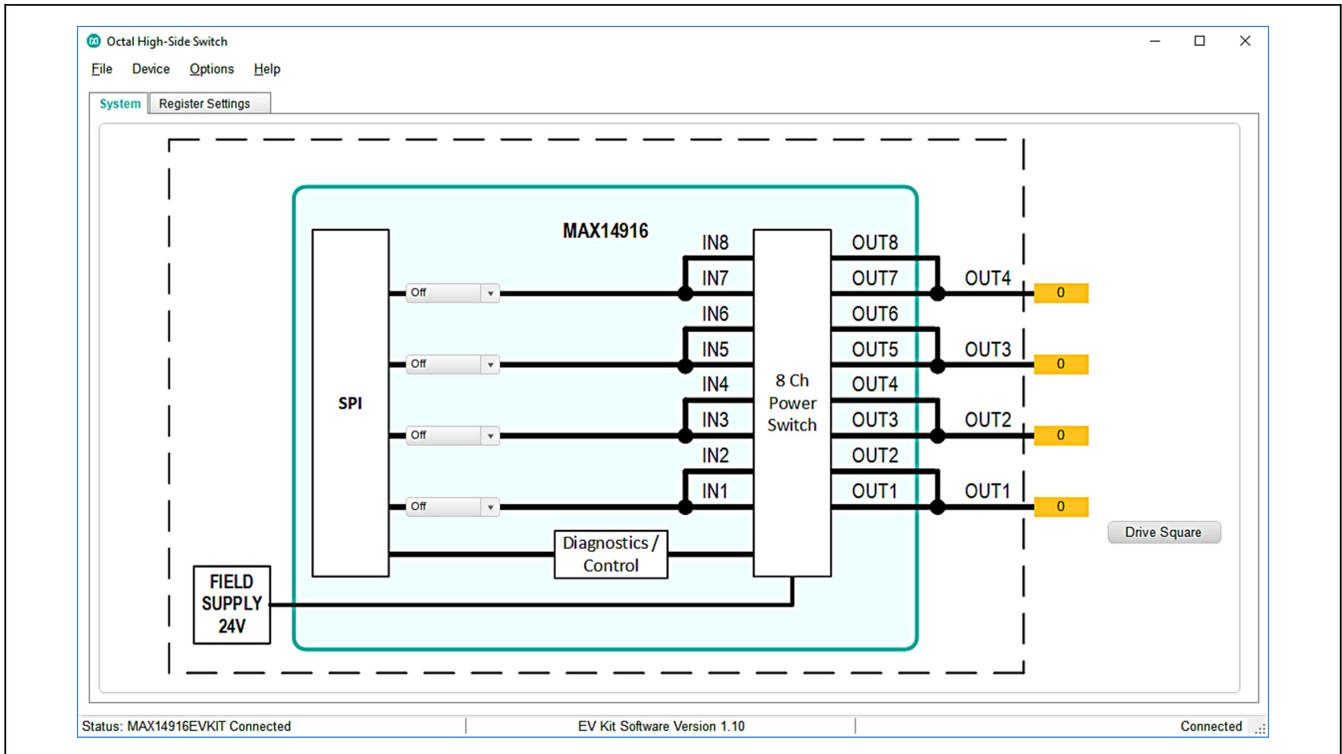
Figure 1. MAX14916 EV Kit GUI System Tab
