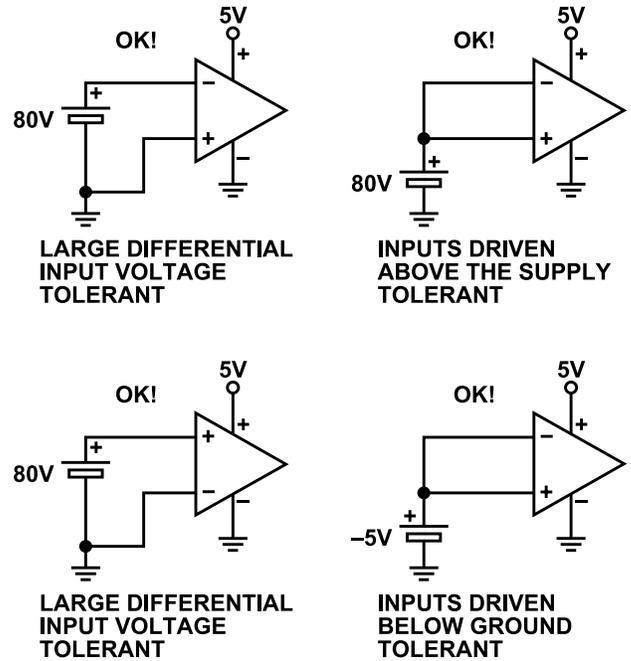
Figure 57. ADA4099-1 and ADA4099-2 Fault Tolerant Conditions
