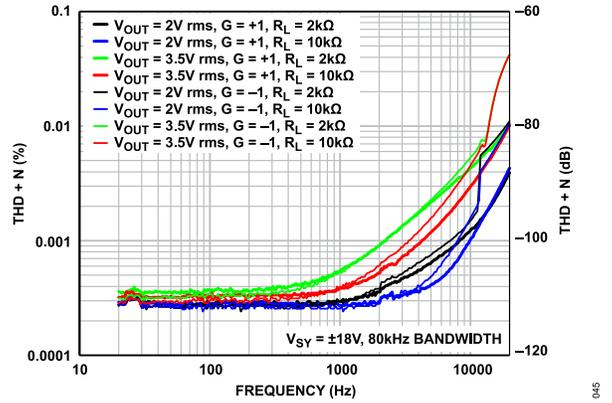
Figure 46. THD + N vs. Frequency over Load
