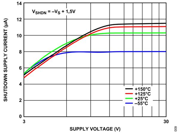
Figure 10. Shutdown Supply Current vs. Supply Voltage
