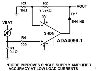
Figure 72. 1 V/A Low-Side Current Sense (ADA4099-1 6-lead TSOT)
