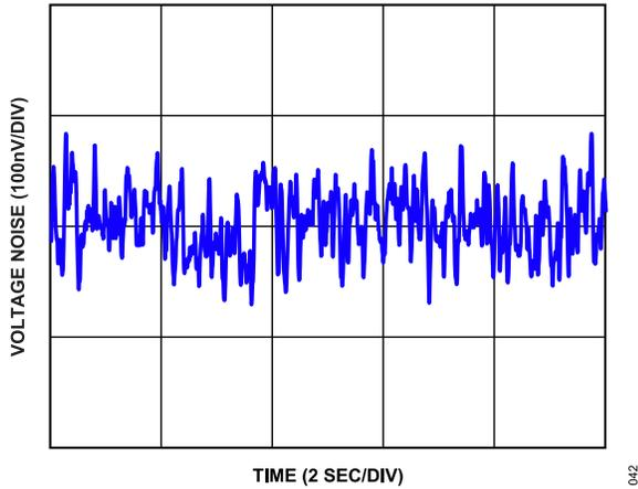
Figure 43. 0.1 Hz to 10 Hz Noise
