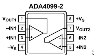
Figure 5. Pin Configuration for ADA4099-2 8-Lead SOIC\_N and 8-Lead MSOP
