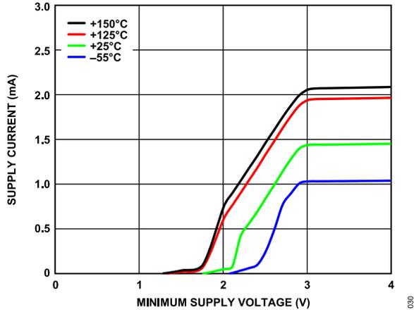
Figure 31. Supply Current vs. Minimum Supply Voltage
