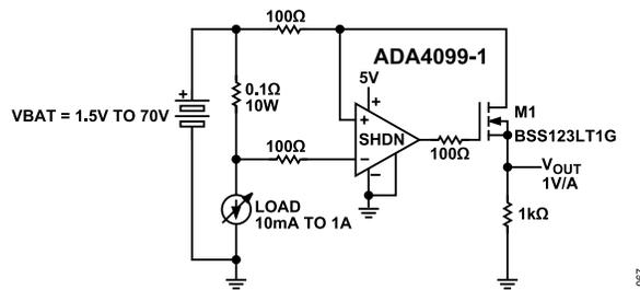
Figure 73. 1 V/A High-Side Current Sense (ADA4099-1 6-lead TSOT)
