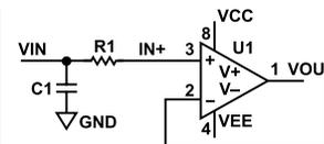
Figure 66. ESD Protection Circuit (RC Network)
