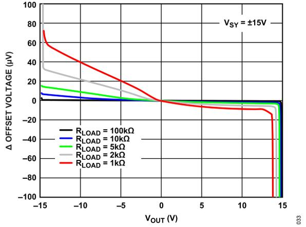
Figure 34. Δ Offset Voltage vs. Output Voltage ( $V_{OUT}$ )
