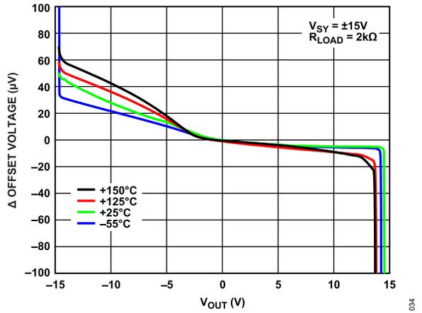
Figure 35. Δ Offset Voltage vs.  $V_{OUT}$  (2 kΩ Load)
