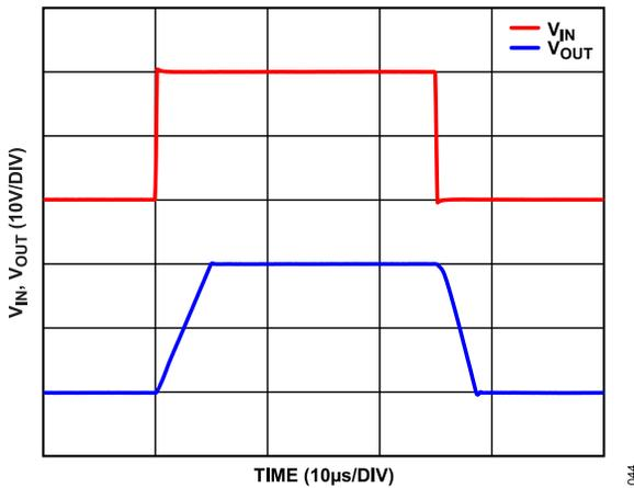
Figure 45. Unity-Gain Large Signal Step Response
