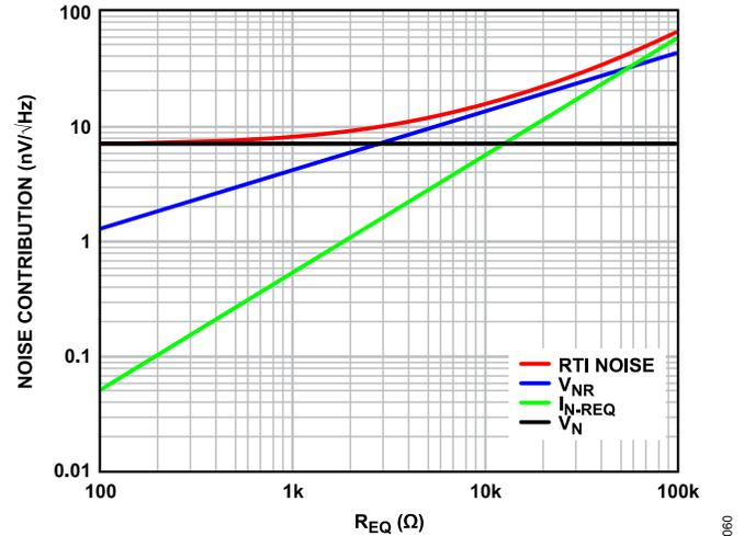
Figure 63. Noise Contributions vs. Equivalent Input Resistance (REQ)
