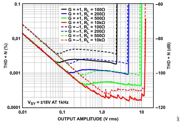
Figure 48. THD + N vs. Output Amplitude and Load
