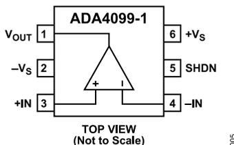
Figure 4. Pin Configuration for ADA4099-1 6-Lead TSOT
