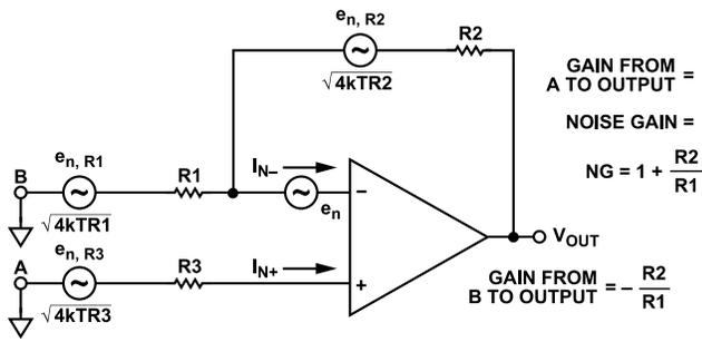
$$RTI\ NOISE = \sqrt{e_n^2 + 4kTR_3 + 4kTR_1 \left(\frac{R_2}{R_1 + R_2}\right)^2 + I_{N+}^2 R_3^2 + I_{N-}^2 \left(\frac{R_1 \times R_2}{R_1 + R_2}\right)^2 + 4kTR_2 \left(\frac{R_1}{R_1 + R_2}\right)^2}$$
