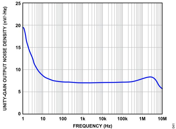
Figure 42. Unity-Gain Output Noise Density vs. Frequency
