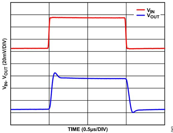
Figure 44. Unity-Gain Small Signal Step Response
