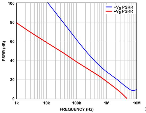
Figure 50. PSRR vs. Frequency
