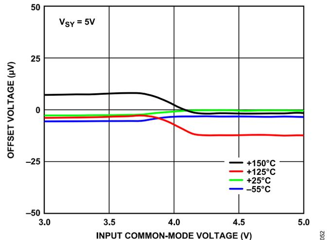
Figure 54. Offset Voltage vs. Input Common-Mode Voltage over Temperature,  $V_{SY} = 5$  V
