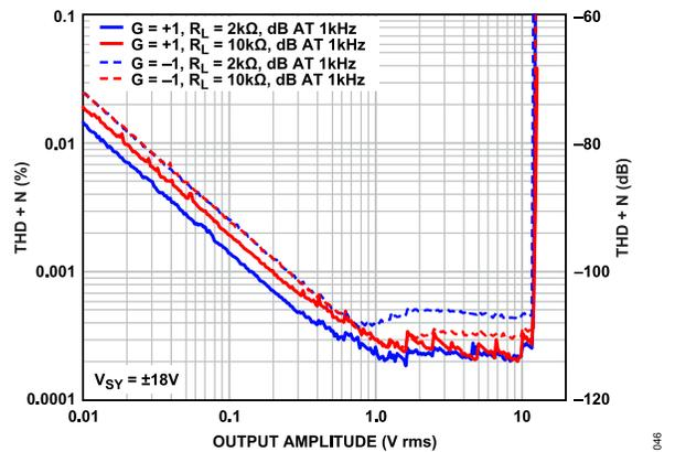
Figure 47. THD + N vs. Output Amplitude
