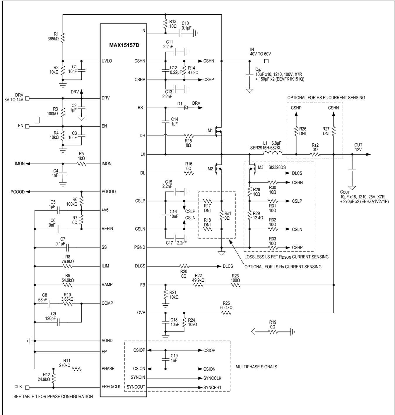
Figure 4. Single-Phase Buck Converter with Lossless LS FET R<sub>DS(on)</sub> Current Sensing
