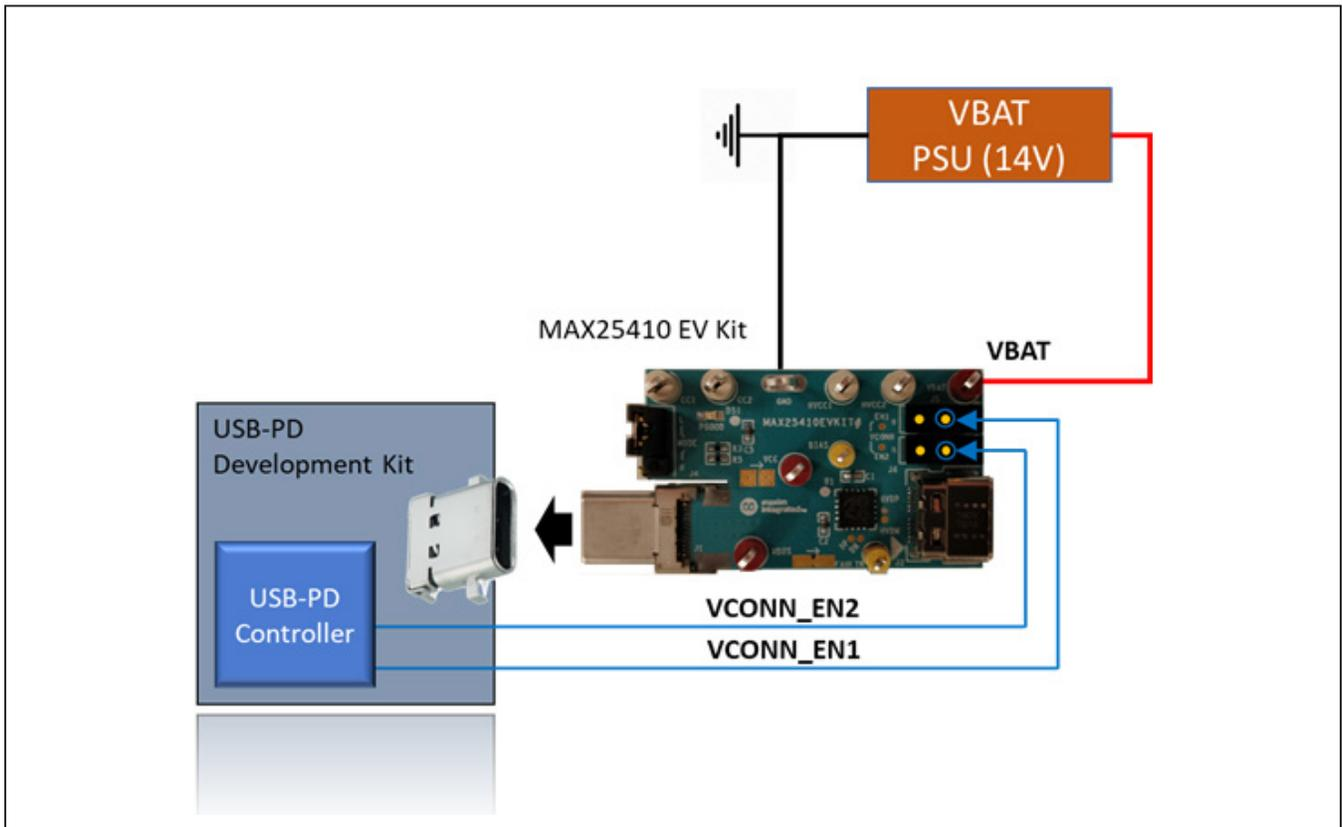
Figure 6. External V<sub>CONN</sub> Control
