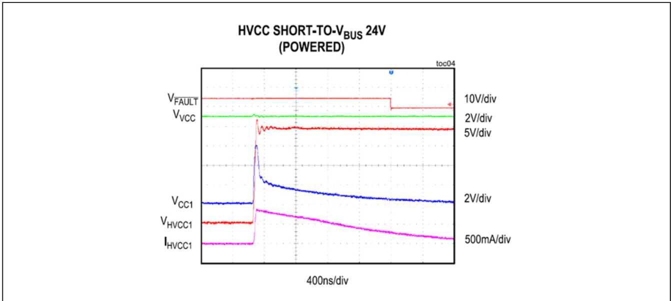
Figure 3. HVCC Short-to-V<sub>BUS</sub> Response
