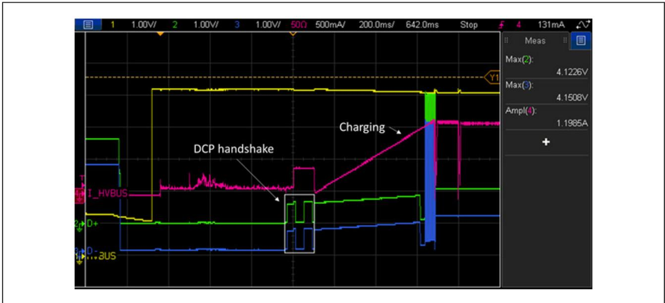
Figure 12. Auto-DCP Response with an Android phone
