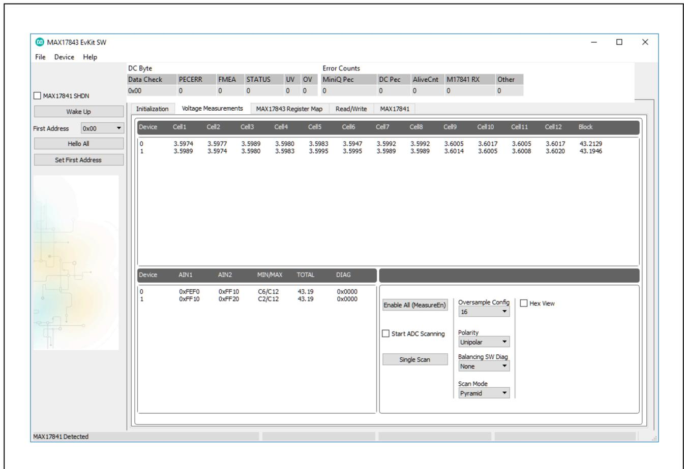
Figure 8. MAX17843 Evaluation Kit Software (Voltage Measurements Tab—Single Scan)
