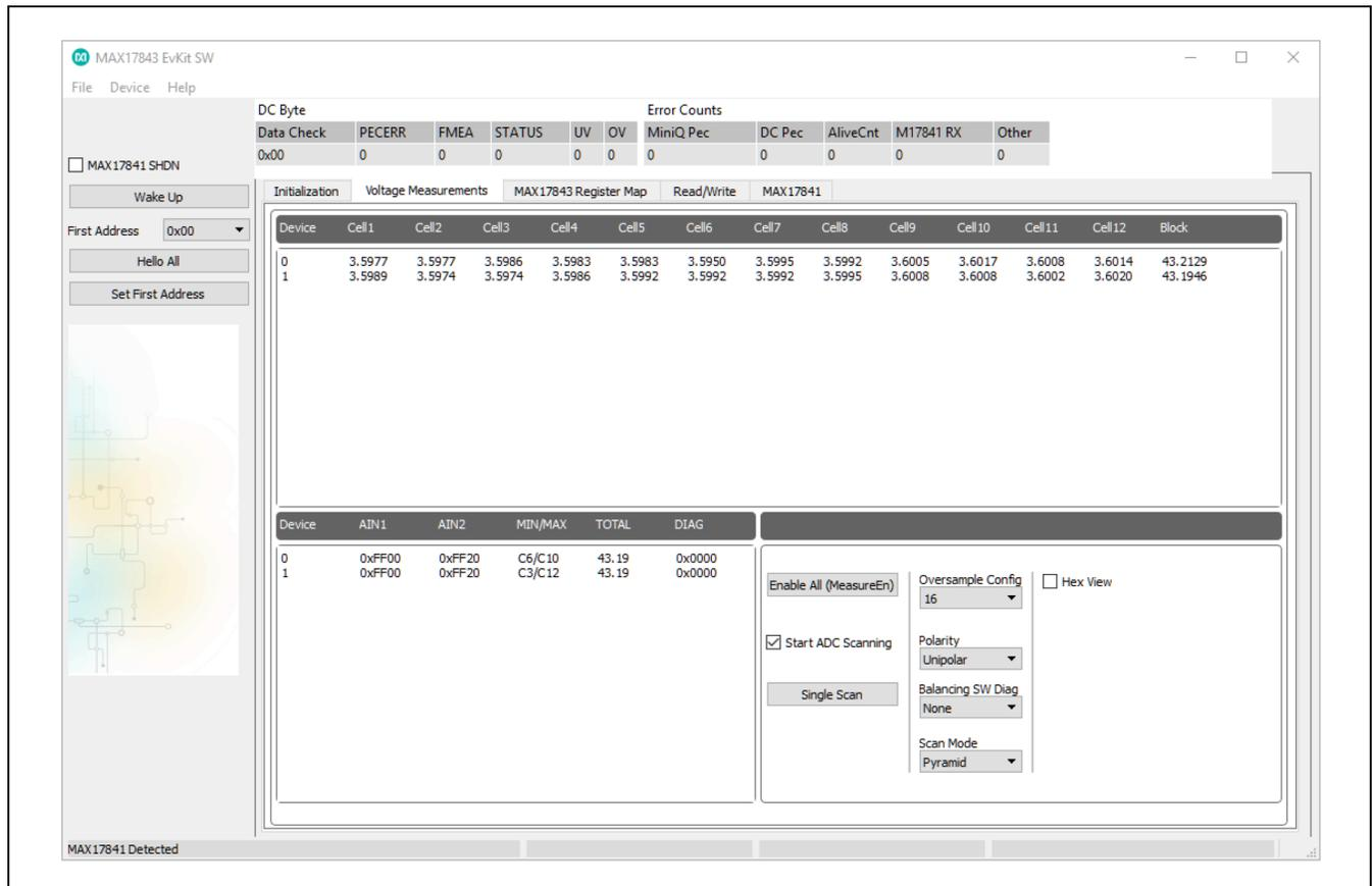
Figure 7. MAX17843 Evaluation Kit Software (Voltage Measurements Tab)
