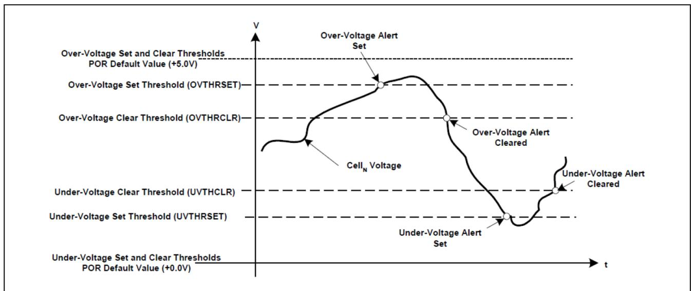
Figure 14. Programmable Overvoltage and Undervoltage Thresholds Diagram
