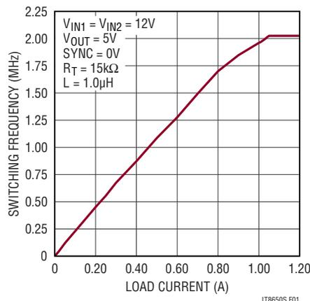
Figure 1. Burst Frequency
