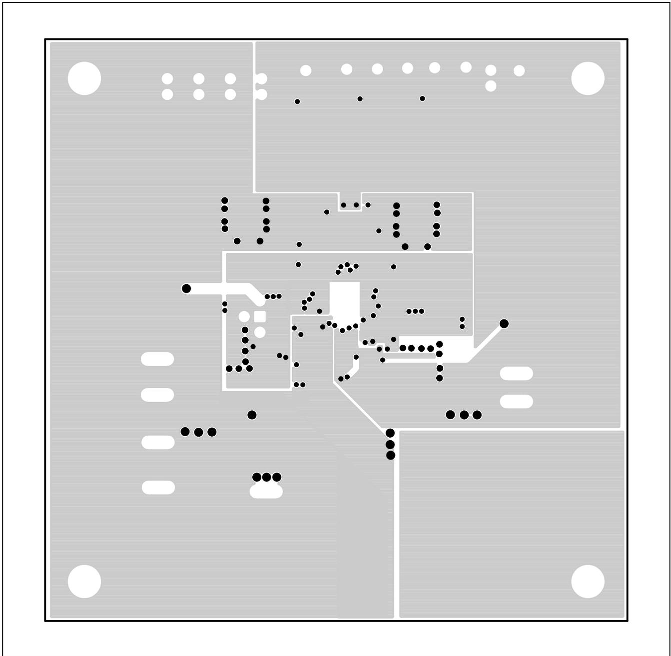
Figure 5. MAX16930 EV Kit PCB Layout—Layer 3 (VIN and AGND)
