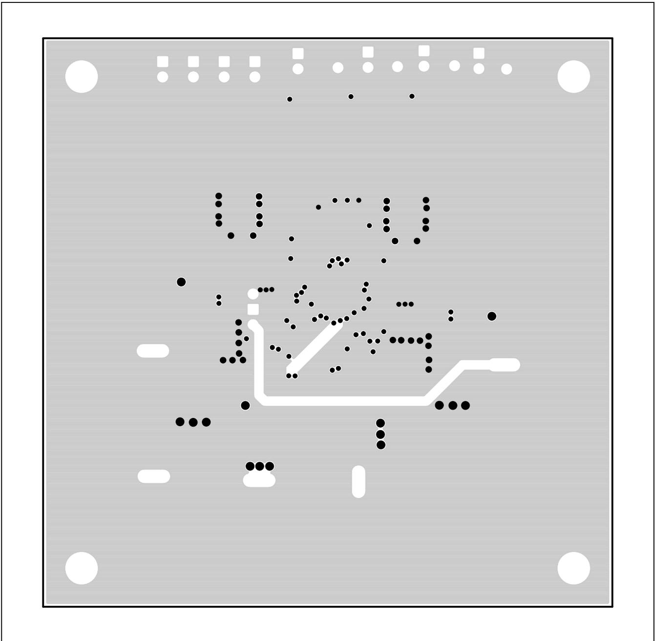
Figure 4. MAX16930 EV Kit PCB Layout—Layer 2 (PGND)
