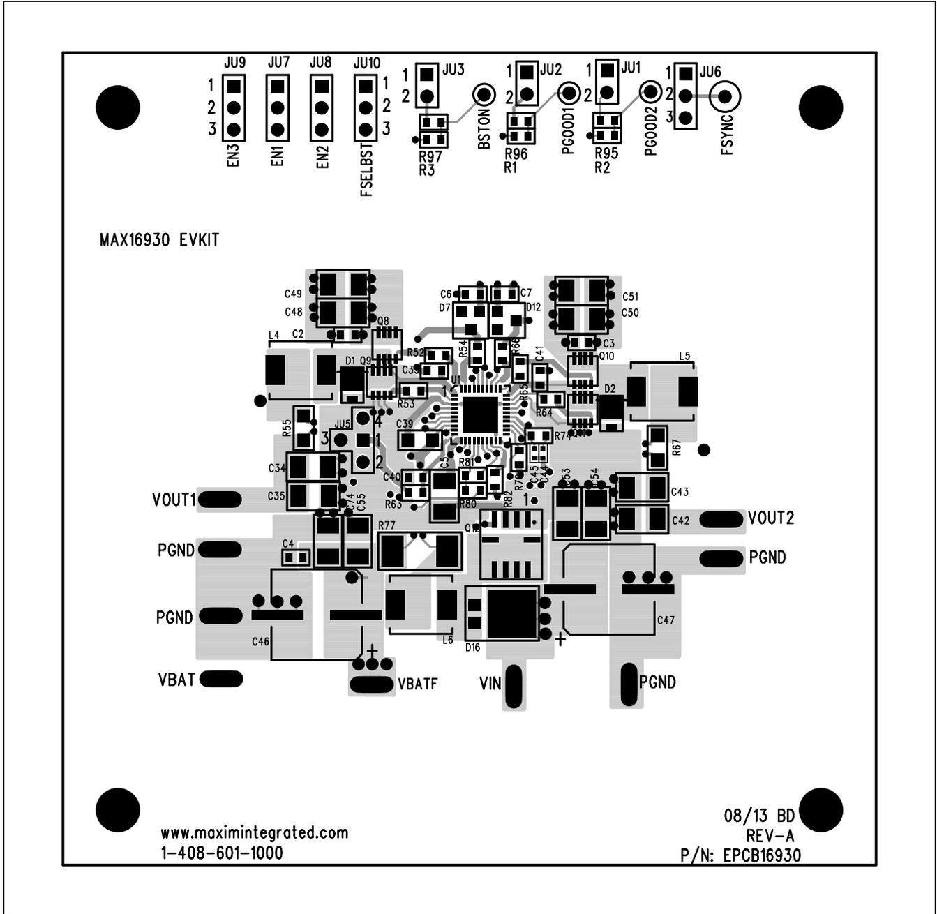
Figure 3. MAX16930 EV Kit PCB Layout—Component Side
