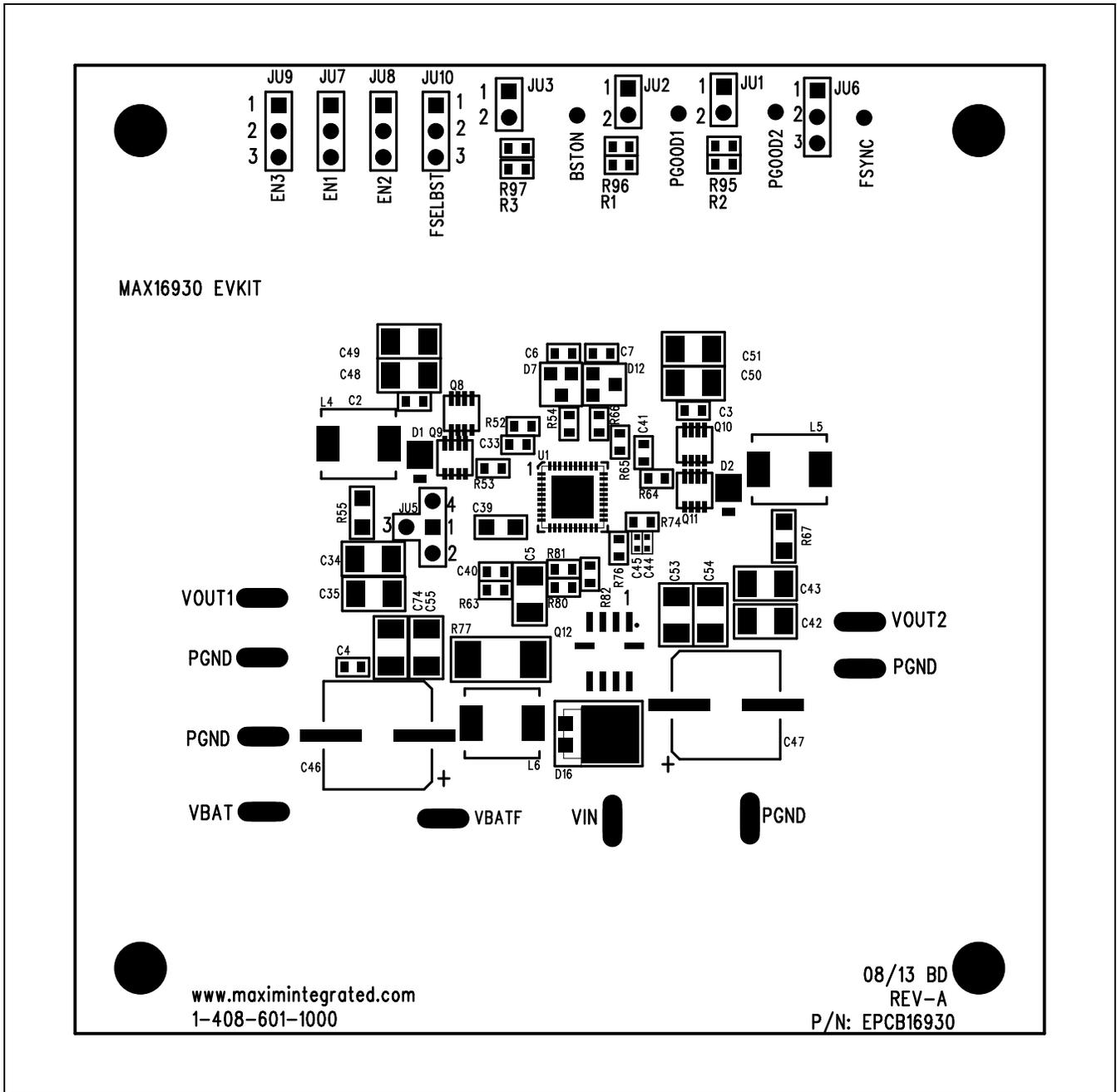
Figure 2. MAX16930 EV Kit Component Placement Guide—Component Side
