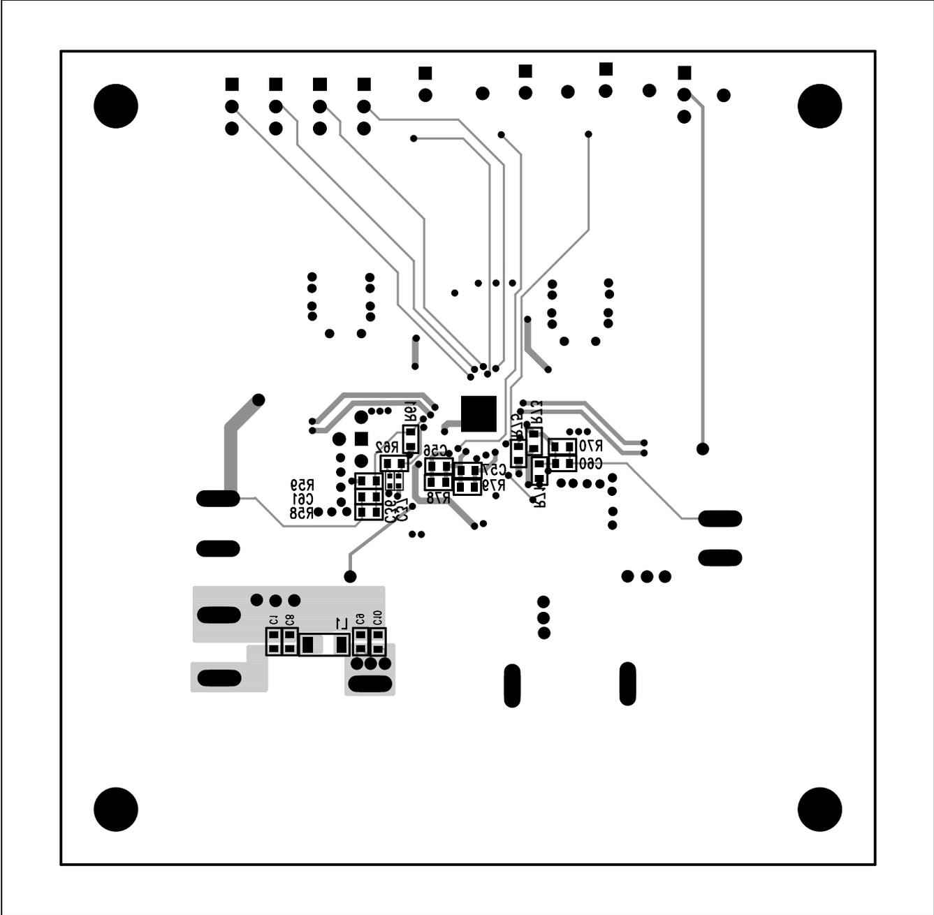
Figure 6. MAX16930 EV Kit PCB Layout—Solder Side
