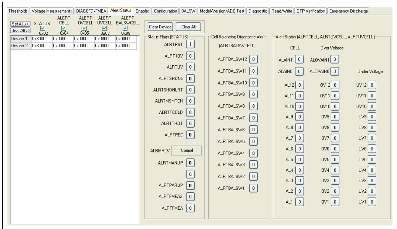
Figure 11. MAX17823 Evaluation Kit Software (Alert/Status Tab)
