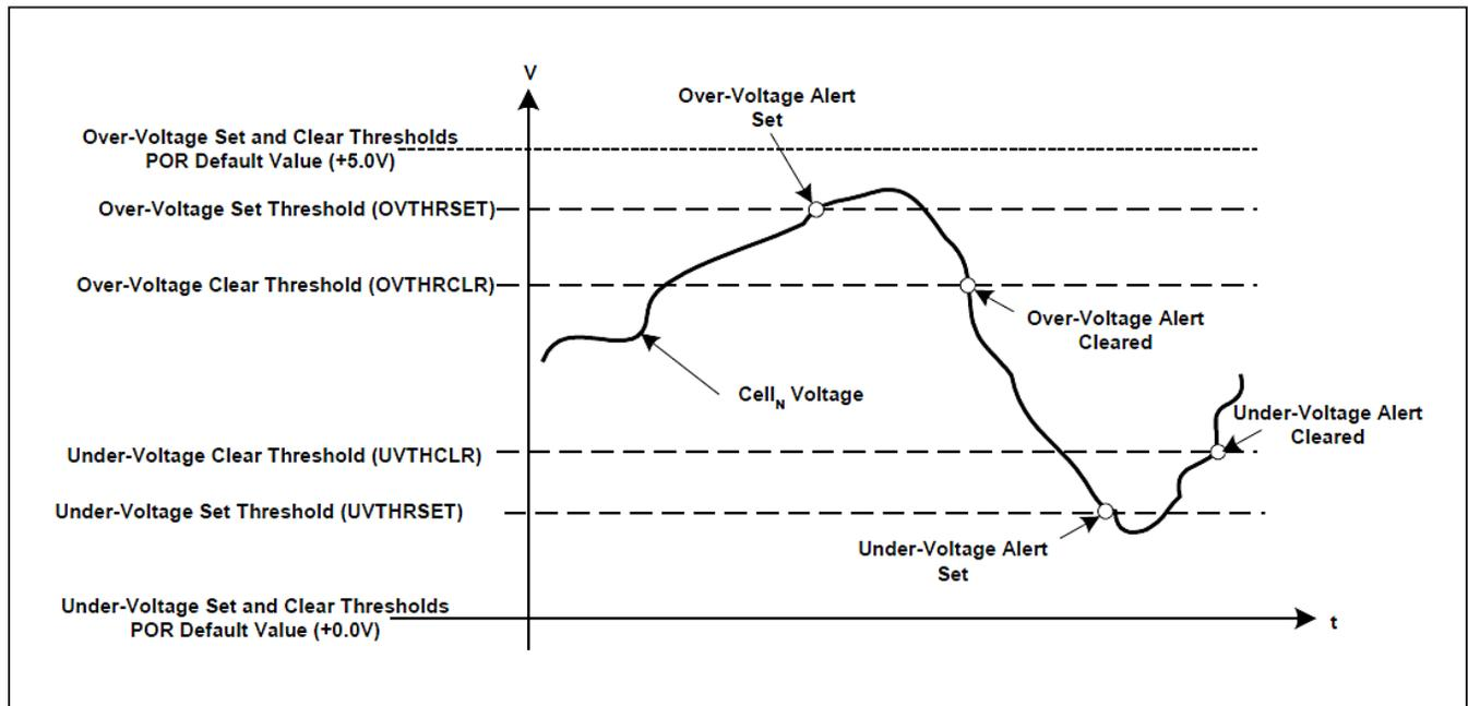
Figure 19. Programmable OV and UV Thresholds Diagram
