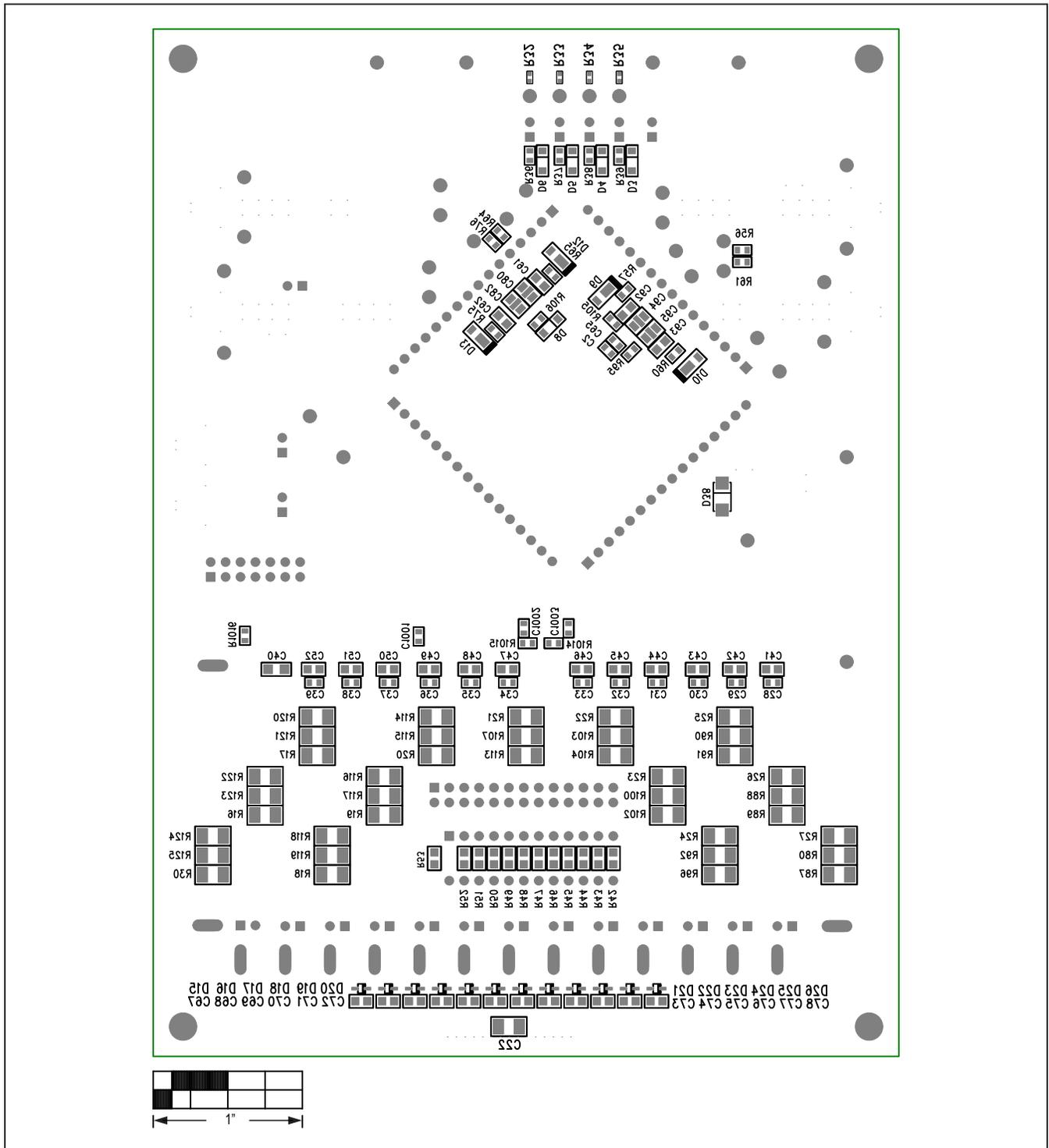
Figure 29. MAX17823 EV Kit PCB Bottom Layer Silkscreen
