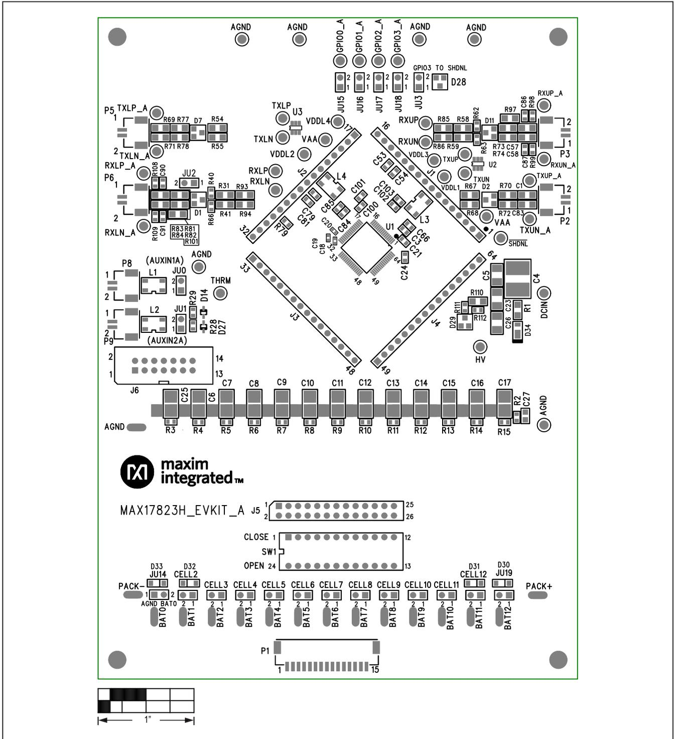
Figure 24. MAX17823 EV Kit PCB Top Layer Silkscreen
