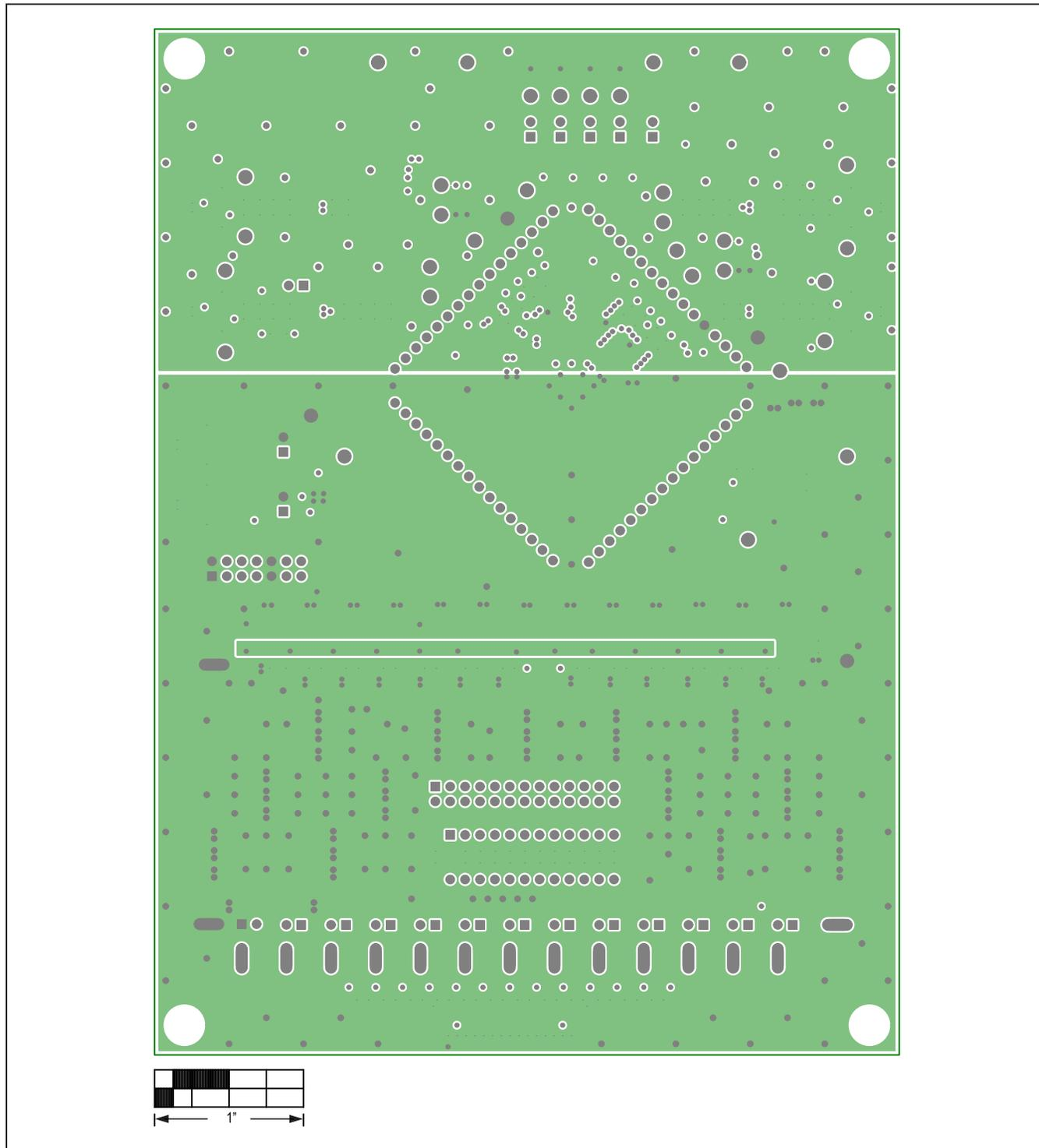
Figure 27. MAX17823 EV Kit PCB Layer Three Metal
