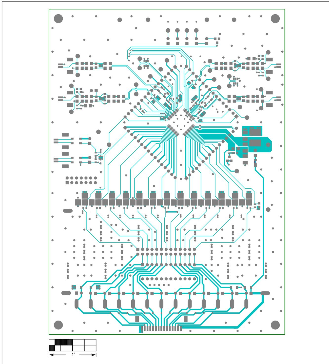
Figure 25. MAX17823 EV Kit PCB Top Layer Metal
