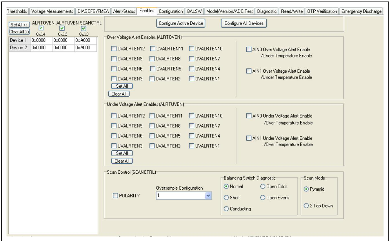
Figure 12. MAX17823 Evaluation Kit Software (Enables Tab)
