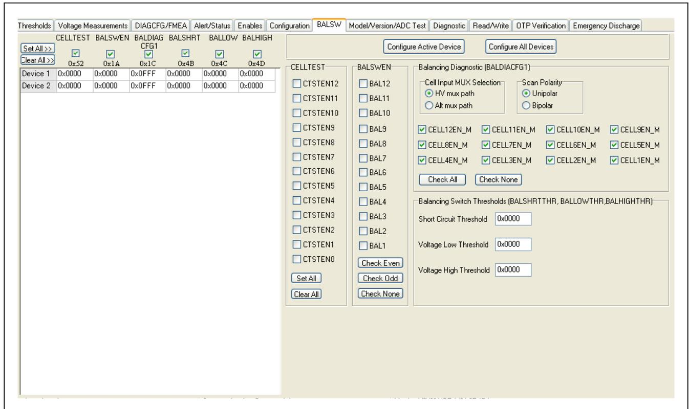
Figure 14. MAX17823 Evaluation Kit Software (Switches Tab)
