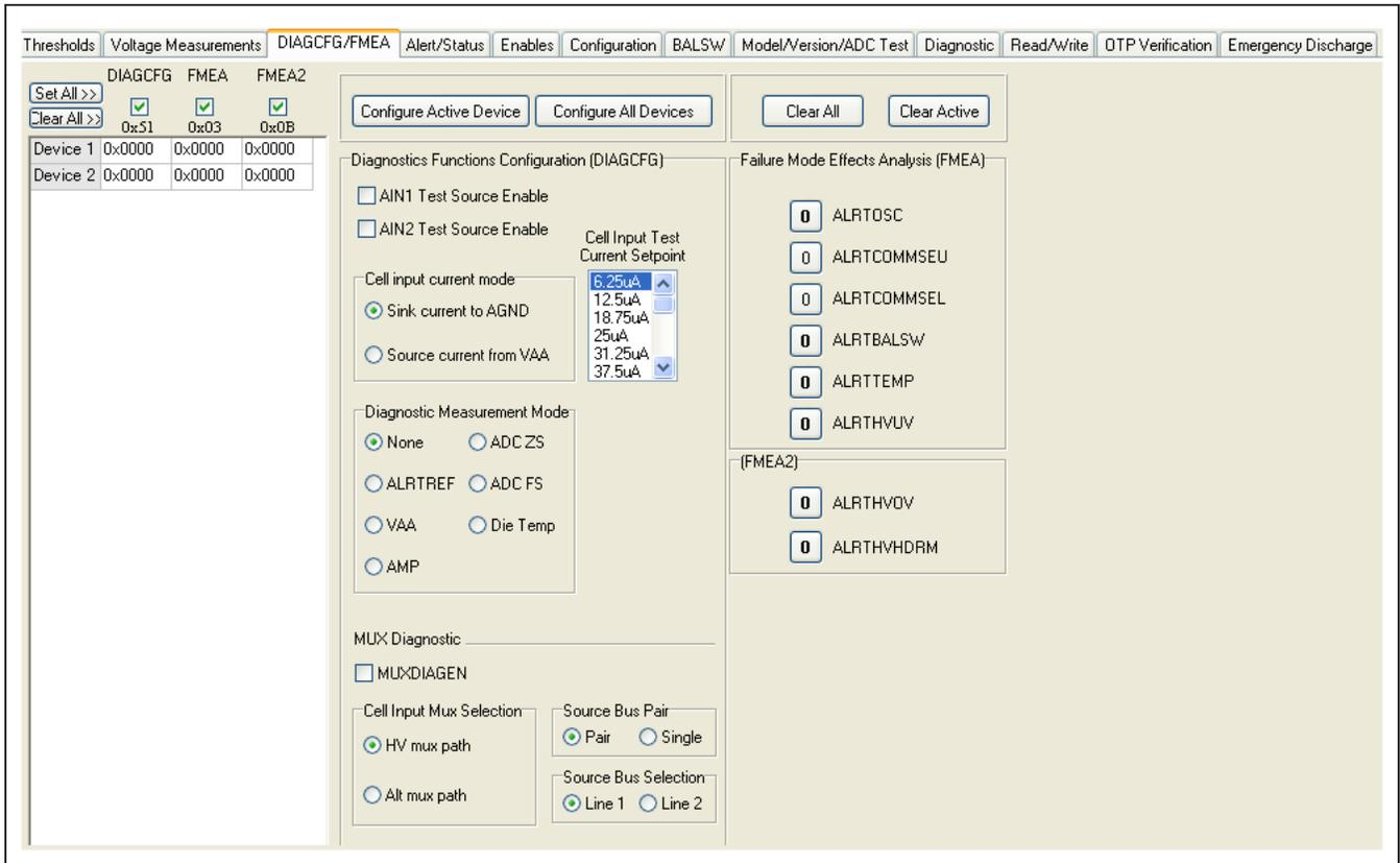
Figure 10. MAX17823 Evaluation Kit Software (DIAGCFG/FMEA Tab)
