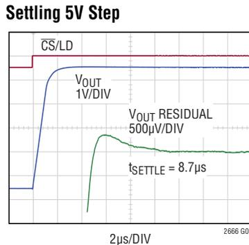
0V TO 5V RANGE; INTERNAL REFERENCE RISING 5V STEP; AVERAGE OF 128 EVENTS FALLING SETTLING IS SIMILAR OR BETTER RESIDUAL WAVEFORM INCLUDES 100ns FIXTURE DELAY
