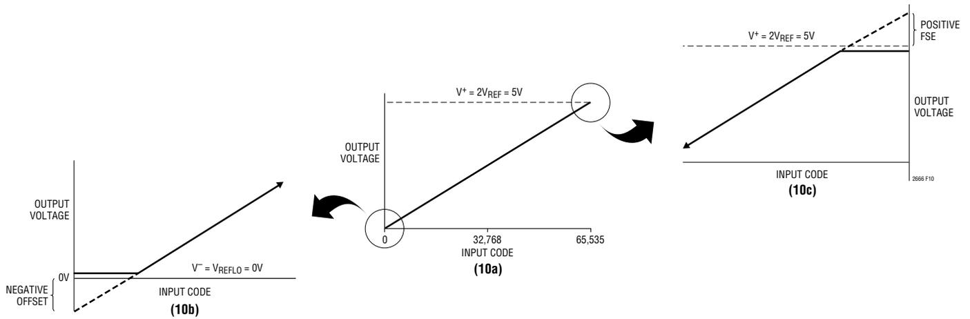
**Figure 10. Effects of 0V to 5V Output Range for Single-Supply Operation. (10a) Overall Transfer Function (10b) Effect of Negative Offset for Codes Near Zero-Scale (10c) Effect of Positive Full-Scale Error for Codes Near Full-Scale**
