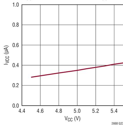
**$V^+/V^-$  Shutdown Current vs Symmetric Supplies**
