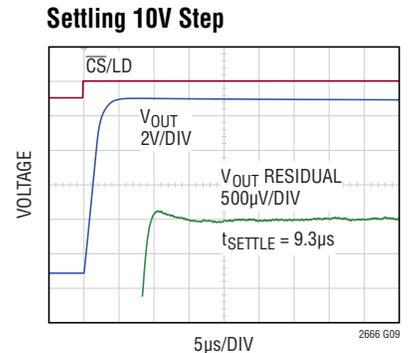
0V TO 10V RANGE; INTERNAL REFERENCE RISING 10V STEP; AVERAGE OF 128 EVENTS FALLING SETTLING IS SIMILAR OR BETTER RESIDUAL WAVEFORM INCLUDES 100ns FIXTURE DELAY
