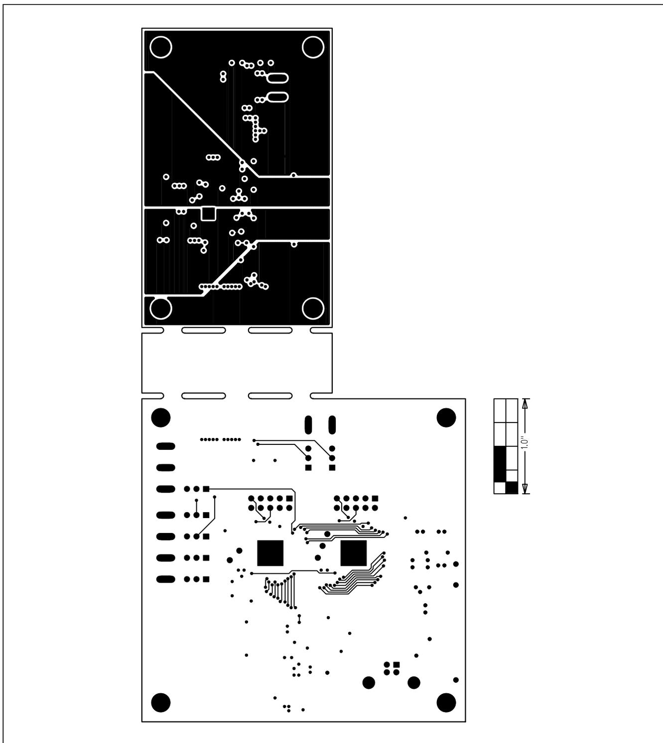
Figure 9. MAX16826 EV Kit PCB Layout—Solder Side
