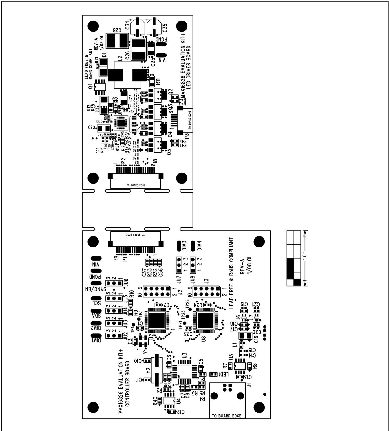
Figure 5. MAX16826 EV Kit Component Placement Guide—Component Side
