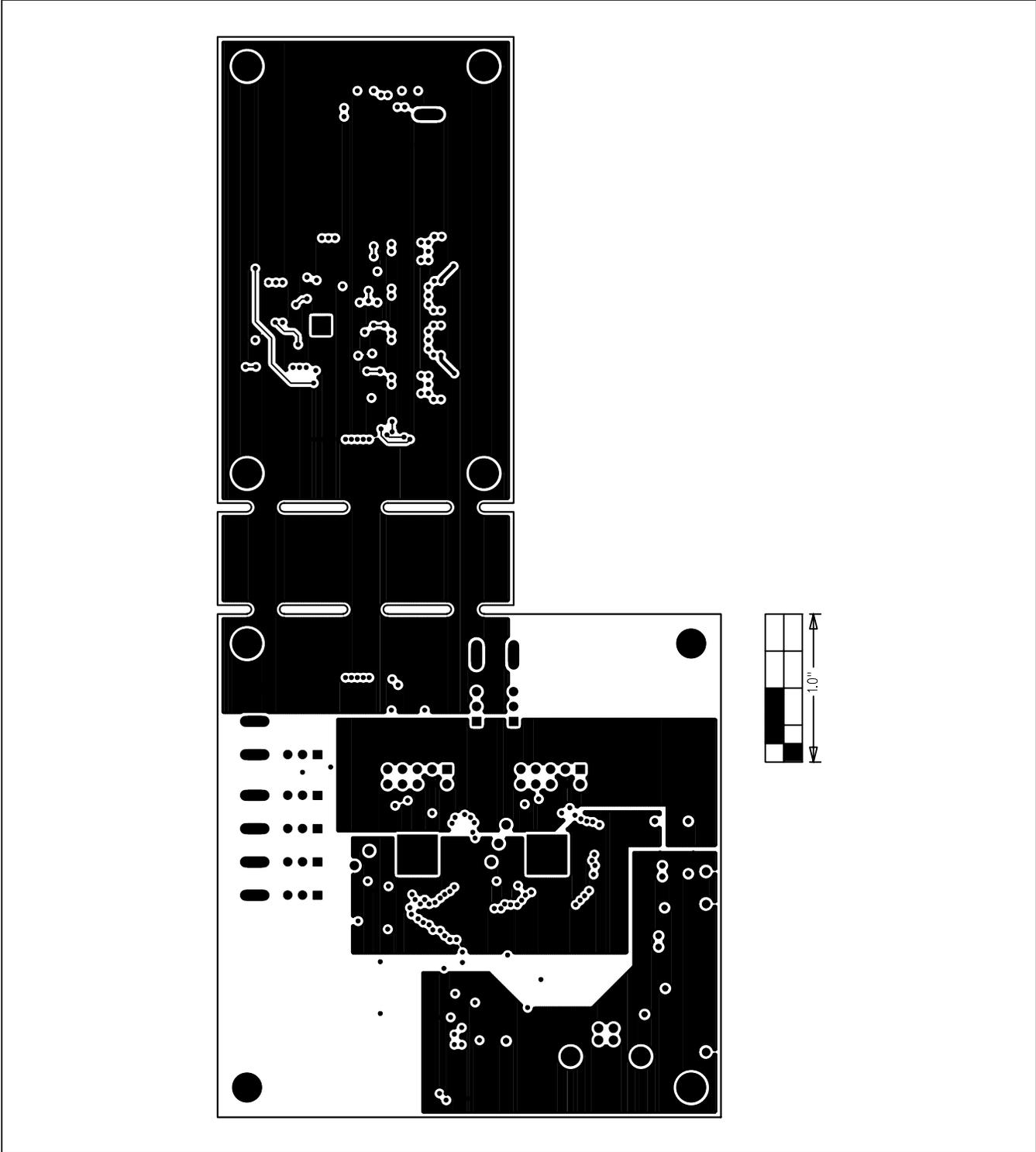
Figure 7. MAX16826 EV Kit PCB Layout—Layer 2
