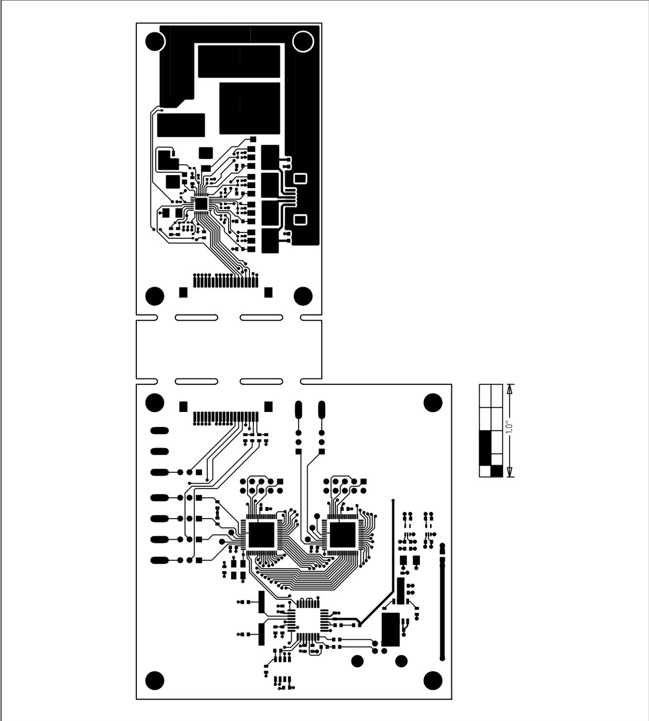
Figure 6. MAX16826 EV Kit PCB Layout—Component Side
