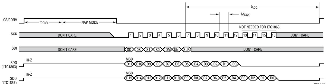
**Figure 6. Example 1,  $\overline{\text{CS}}/\text{CONV}$  Starts a Conversion and Remains HIGH Until Next Data Transfer. With  $\overline{\text{CS}}/\text{CONV}$  Remaining HIGH After the Conversion, Automatic Nap Modes Provides Power Reduction at Reduced Sample Rate**
