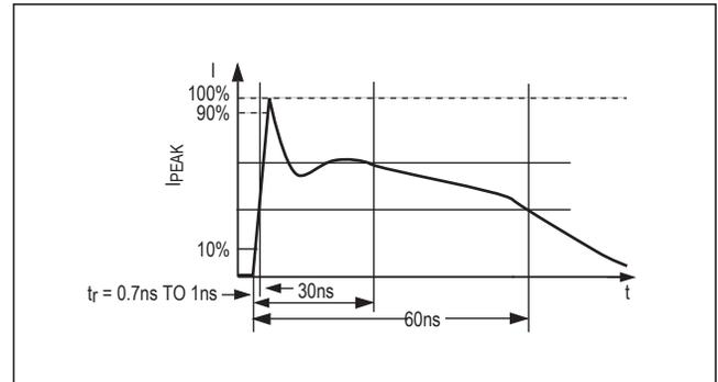
Figure 11. IEC 61000-4-2 ESD Generator Current Waveform
