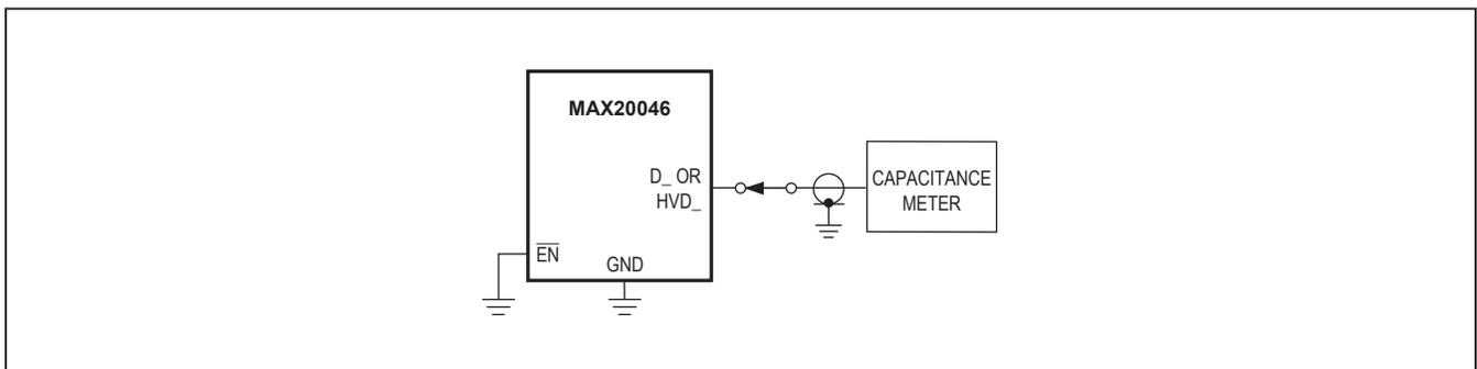
Figure 6. On-Capacitance
