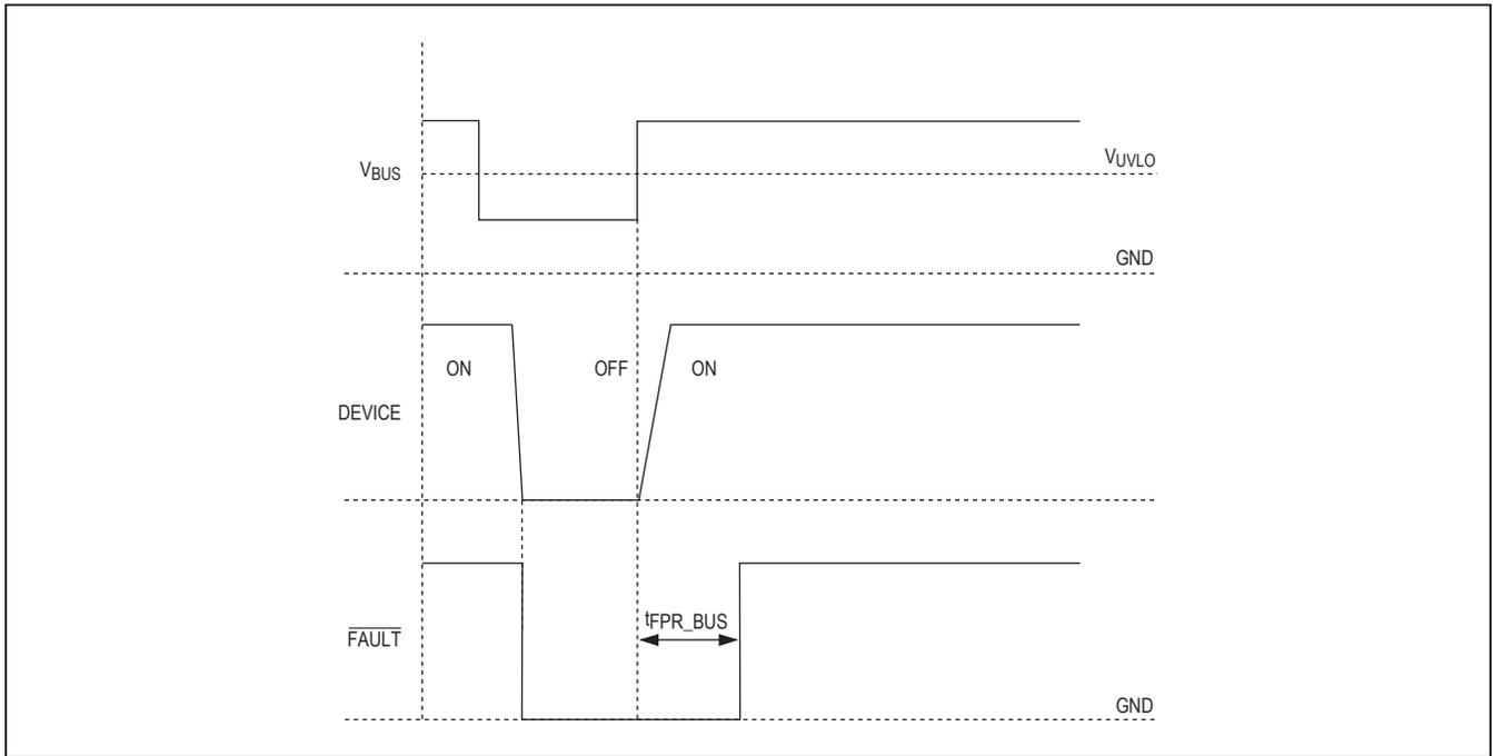
Figure 1. Timing Diagram for Undervoltage Lockout on BUS
