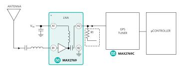
Figure 2. GPS Receiver Front-End Circuitry
