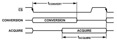
Figure 3. Internal Conversion Acquire Timing
