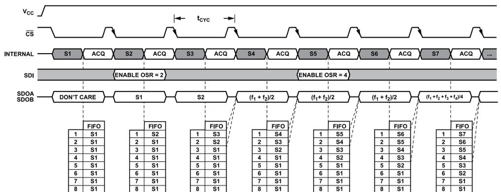
Figure 36. Rolling Average Oversampling Mode Configuration
