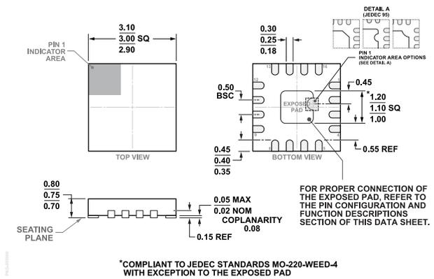
Figure 47. 16-Lead Lead Frame Chip Scale Package [LFCSP]
