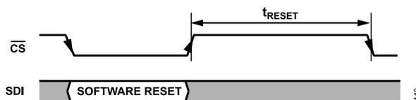
Figure 38. Software Reset Operation
