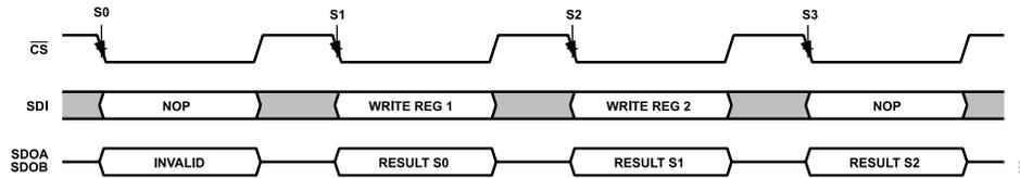
Figure 45. Register Write
