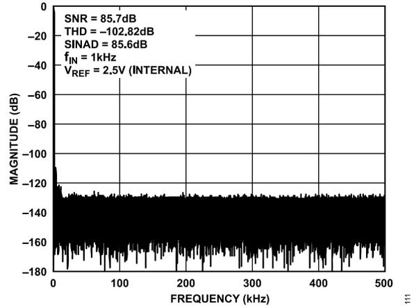
Figure 10. AD4682 FFT,  $V_{REF} = 2.5\text{ V}$  Internal
