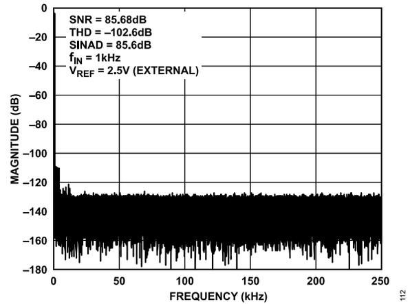
Figure 11. AD4683 FFT,  $V_{REF} = 2.5\text{ V}$  External
