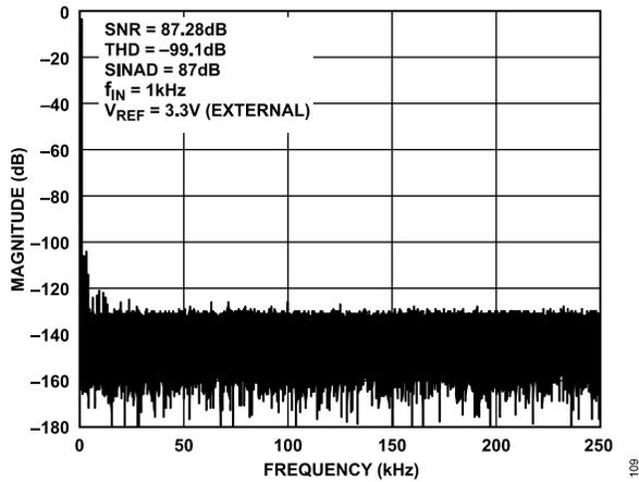
Figure 8. AD4683 FFT,  $V_{REF} = 3.3\text{ V}$  External
