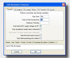
Alternately, if you are only interested in a few node voltages and device currents, you can restrict the quantity of saved data by using the .save directive to save only those specific node voltages and device currents. In the directive, add the "dialogbox" option to display all available nodes and currents so you can choose to save additional data of interest.
