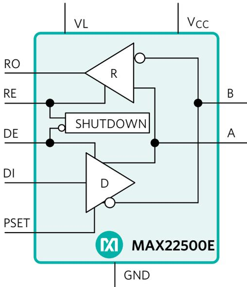
Figure 2. Functional Diagram of the MAX22500E
