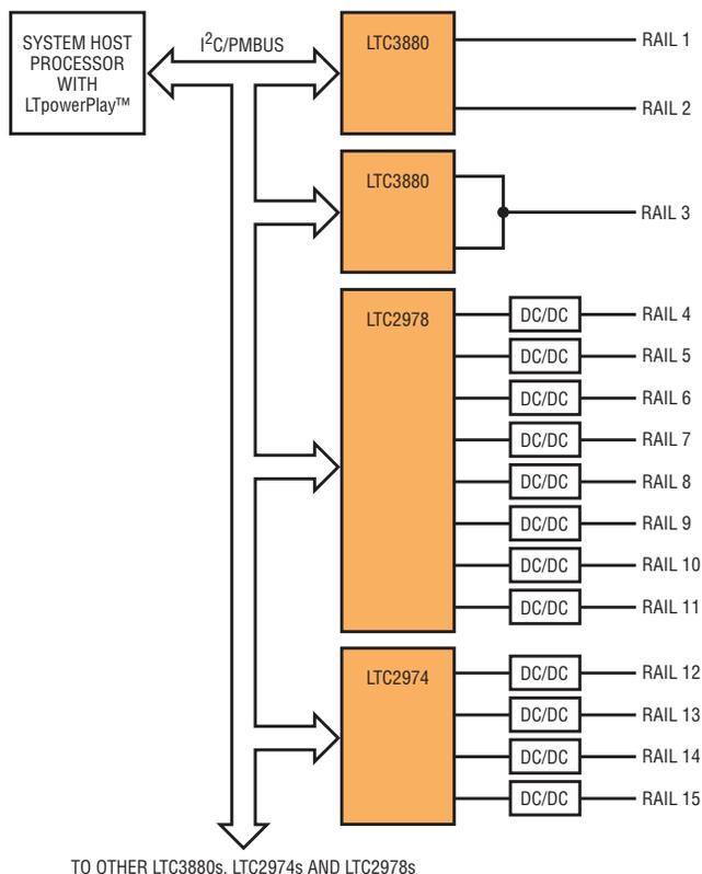
Linear Technology PMBus controllers such as the LTC3880 and companion ICs such as the LTC2978 make it easy to program power-up and power-down sequencing for any number of supplies. By using a time-based algorithm, users can dynamically sequence rails on and off in any order with simple programmable delays.
