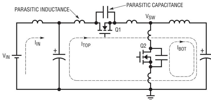
Figure 3. Typical switch node voltage spike and ringing in a 12V input buck switching regulator
