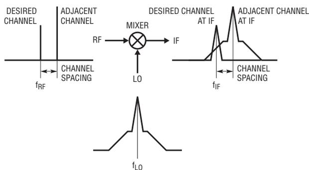
Figure 6. Reciprocal mixing due to LO phase noise
