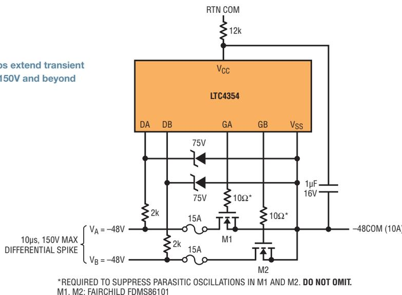
Zeners in the 250mW to 500mW range are capable of absorbing the peak current generated by a 150V, 10μs spike. Higher voltage and longer duration spikes may be accommodated by larger devices.
