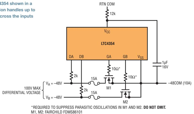
If it were possible to further increase the series resistance, even higher voltages could be tolerated by simply changing the 2k resistor. Unfortunately the drain pin input bias current sets a practical limit of 2k, so as to avoid interfering with the operation of the ideal diode function itself.
