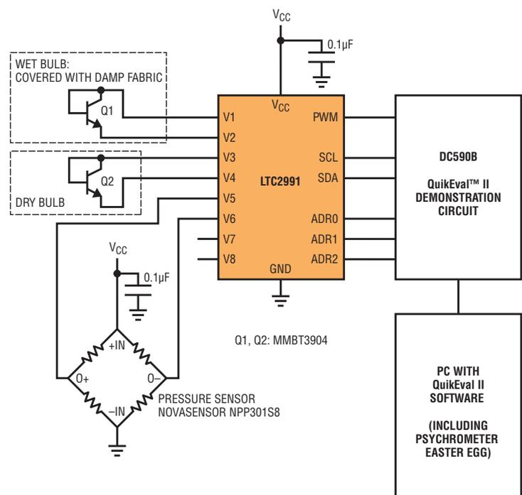
An inexpensive NPN transistor is an ideal temperature sensor for applications calling for disposable sensors, or those that require a large number of sensors.
