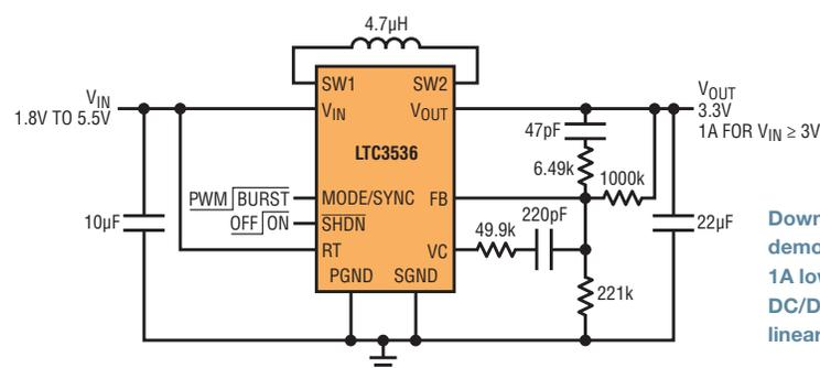
Download the LTspice IV demonstration circuit for this 1A low noise, buck-boost DC/DC converter at [www.linear.com/3536](http://www.linear.com/3536)
