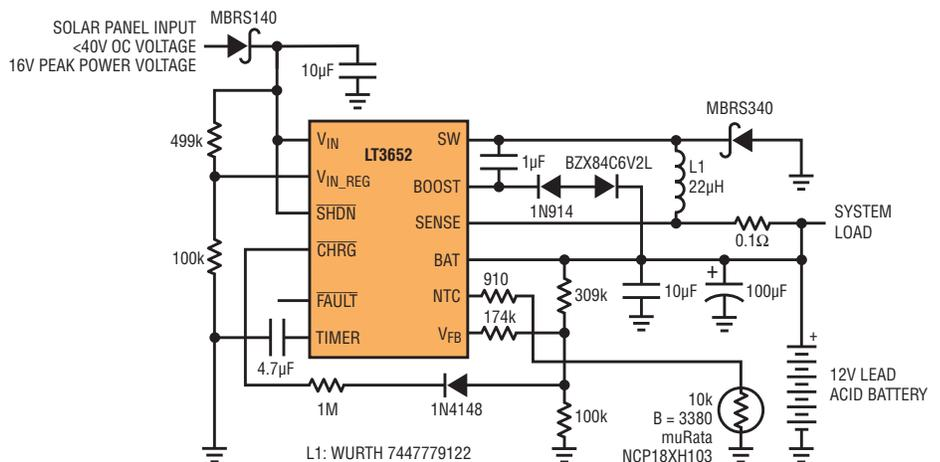
The LTspice IV demonstration circuit for this 1A solar-panel-powered 3-stage 12V lead-acid fast/float charger is available at [www.linear.com/3652](http://www.linear.com/3652)
