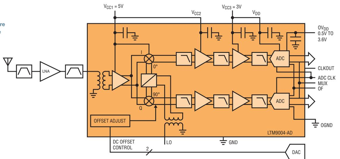
The LTM9004 is a direct conversion receiver utilizing an I/Q demodulator, baseband amplifiers and a dual 14-bit, 125MSPS ADC. The LTM9004-AC lowpass filter has a 0.2dB corner at 9.42MHz, allowing four WCDMA carriers.
