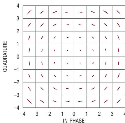
Figure 4. 64-QAM constellation corrupted by phase noise
