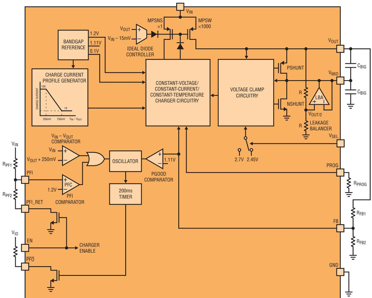
The maximum working voltage on a single supercapacitor is 2.7V or less. Because most systems require operating voltages higher than this, many supercapacitors are supplied as a pair of capacitors within a single, center-tapped package. The LTC4425 is designed to charge stacked supercapacitors and provide a regulated output voltage for the system load.
