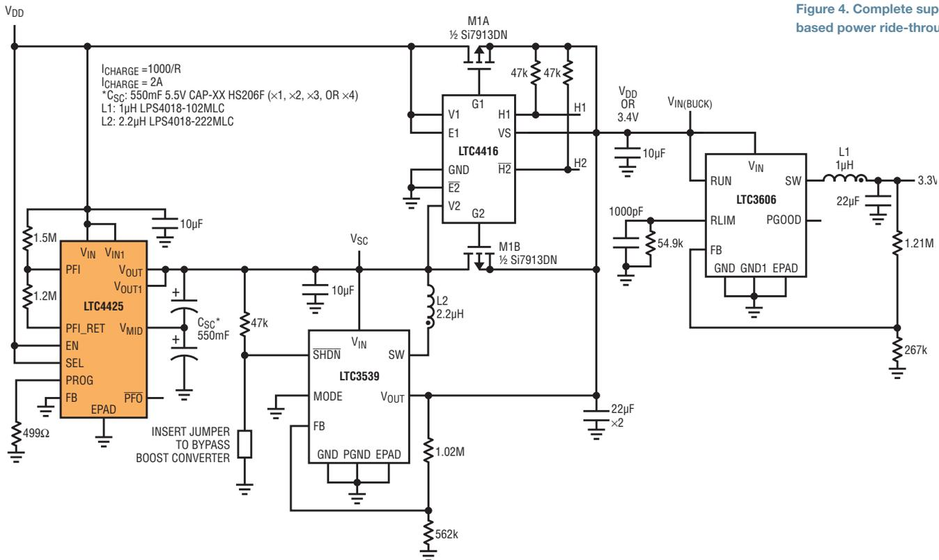
Figure 4. Complete supercapacitor-based power ride-through system
