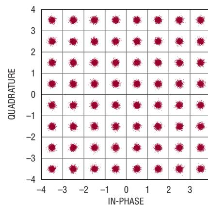
Figure 5. 64-QAM constellation corrupted by white noise
