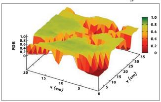
▲ Fig. 3 Multipath fading causes the quality of a link to vary dramatically, even when moving the receiver by only a couple of centimeters.
