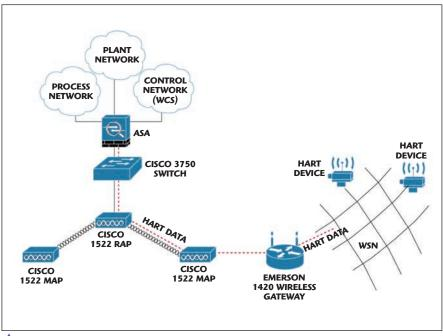
Fig. 6 Network architecture for refinery process control.
