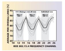
Fig. 2 Interference between Wi-Fi and 802.15.4 in the 2.400 to 2.485 GHz frequency band.
