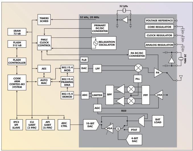
▲ Fig. 5 Block diagram of the LTC5800 Dust Eterna motes.
