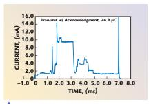
▲ Fig. 1 Energy to transmit a short 802.15.4 packet and receive an acknowledgment.
