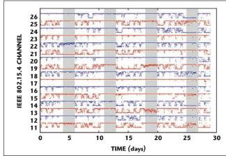
Fig. 4 The packet delivery ratio of a wireless link evolves over time.
