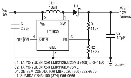
Figure 4. 5V to 12V Boost Converter
