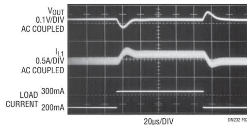
Figure 3. 3.3V to 5V Boost Converter Transient Response
