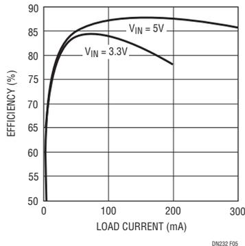
Figure 5. 5V to 12V Boost Converter Efficiency
