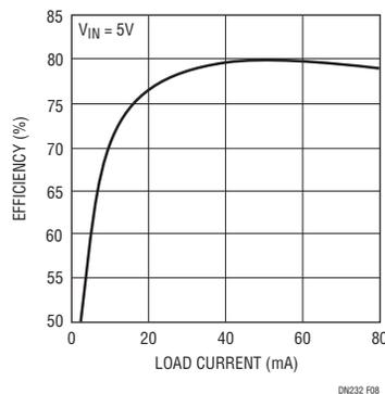
Figure 8. ±15V Dual Output Converter Efficiency
