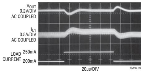
Figure 6. 5V to 12V Boost Converter Transient Response
