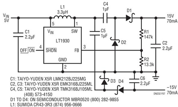
Figure 7. ±15V Dual Output Converter with Output Disconnect
