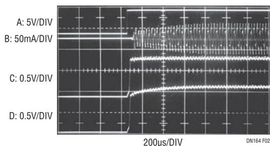
**Figure 2. Fast Loop Response Maintains Regulation at 200Hz PWM Rate. Waveforms Include PWM Command (A), Lamp Current (B), LT1371 Feedback (C) and Error Amplifier V<sub>C</sub> (D) Pins. Loop Settling Occurs in 500µs**
