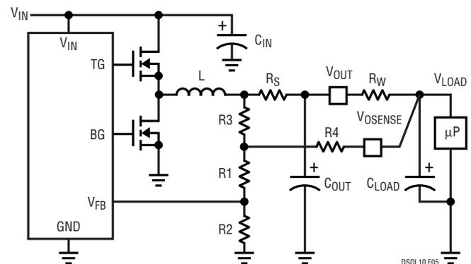
Figure 5. Simplified Buck Regulator with Remote Sense
