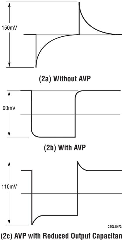
Figure 2. Transient Response Comparison
