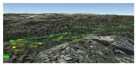
Wireless sensor network installed at Duncan Peak in the Sierra Nevada mountains. Sierra\*net (http://systems.berkeley.edu/wsn/), an initiative between UC Berkeley and UC Merced, is aimed at studying mountain hydrology and improving the forecasting and control of water supplies by using SmartMeshenabled sensors.
